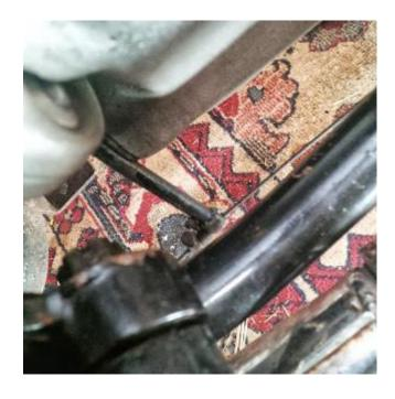
Actuating lever fouling the gearbox housing
