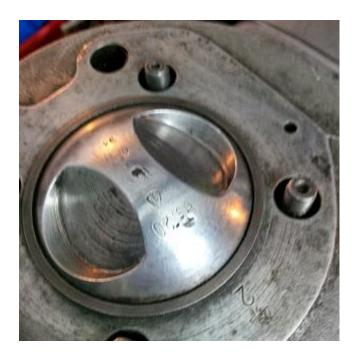
Cleaned up piston ready for head to go back on
