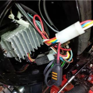
Push fit Battery lead terminals securely mounted Solid state box securely attached to box lid with industrial Velcro Trickle charger socket wired in
